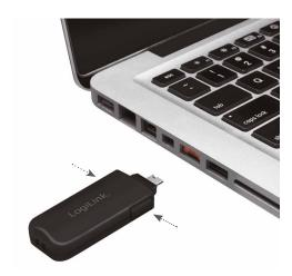
Push the button backwards and pull out the Key. The USB-C port is locked.
